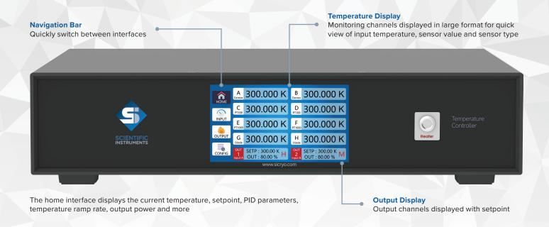
The TC-8 Cryogenic Temperature Controller is engineered for precision and versatility in low-temperature research applications. It features eight independent, high-accuracy temperature monitoring channels, providing robust and reliable measurement capabilities. The unit includes two high-power, PID-controlled output channels (100 W and 50 W), enabling efficient and stable thermal regulation.
